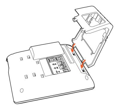
B. Press the other side joints into the slot according to the direction of the arrow:
