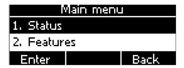
Move the navigation key and press the softkey "**Enter**" or input the corresponding Number key Select the item of Main Menu:
