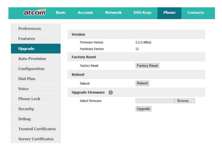
Before upgrading the firmware of phone, users are suggested to check the version of current firmware. Click the button "Choose file" to select the target local file and click "Upgrade" to process upgrading, this will cost a couple of minutes. And after reboot, the phone will be upgraded successfully.
