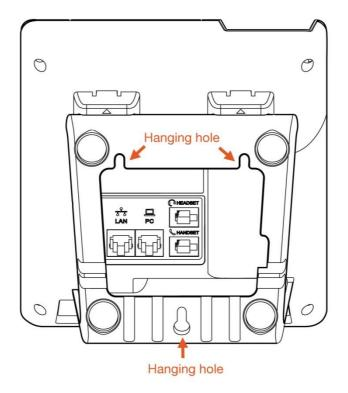
F. It is the right picture after fixing the stand bracket below:
