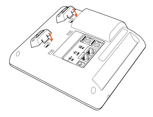
C. After install the wall-hung stand bracket, press one-sidejoints of stand bracket into the slot, please refer to the picture as below:
