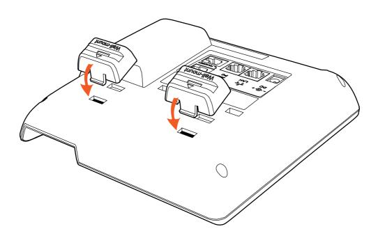
$\ensuremath{\mathsf{B}}.$  Press the other side joints into the slot according to the direction of the arrow
