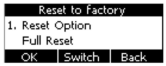
Reset Option: Full Reset, Config Reset and UserData Reset.
