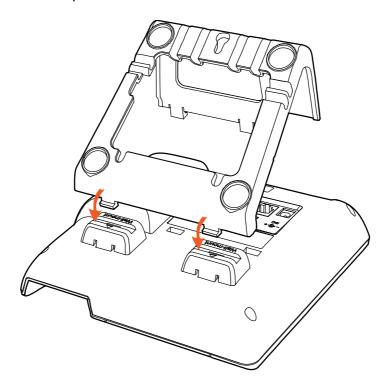
D. Press the other side joints into the slot according to the direction of the arrow
