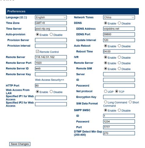
The preference page shown above consists of the following system level parameters and options as shown in the table below.
