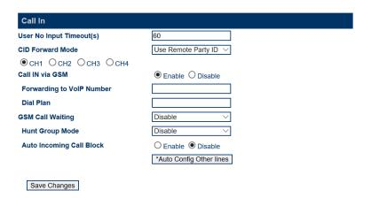
There are two types of parameters. The parameters above the Channel Selection © CH1 O CH2 O CH3 O CH4 are for all channels and the parameters listed below it are for the selected channel only.
