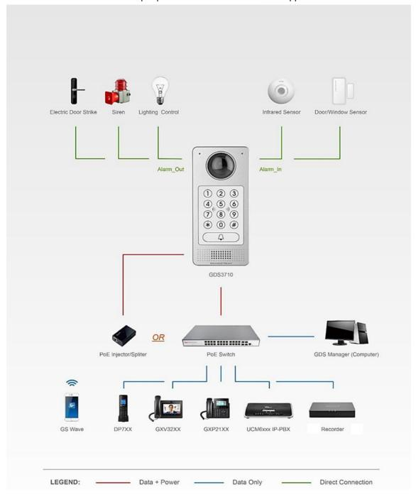
Figure 17: Peripheral Connections for GDS3710
