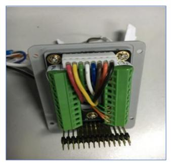
Figure 115: Wiegand Interface Cable
