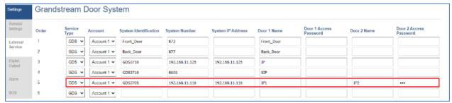
Figure 43: GSC3570 Configuration Example
