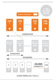
One Hardware for all functions: N870 IP PRO appliance. Function is set by role in the device settings: Integrator, DECT Manager and/or Base station.
