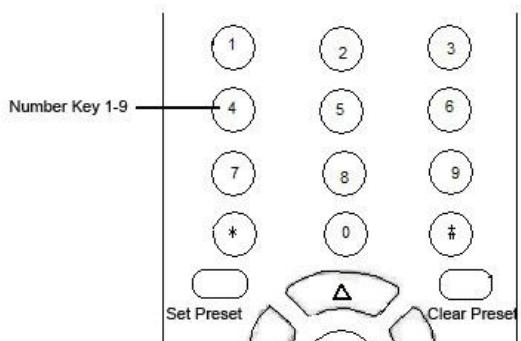
1、Preset setting : to set a preset position, the users should press the "【SET PRESET】" key first and then
