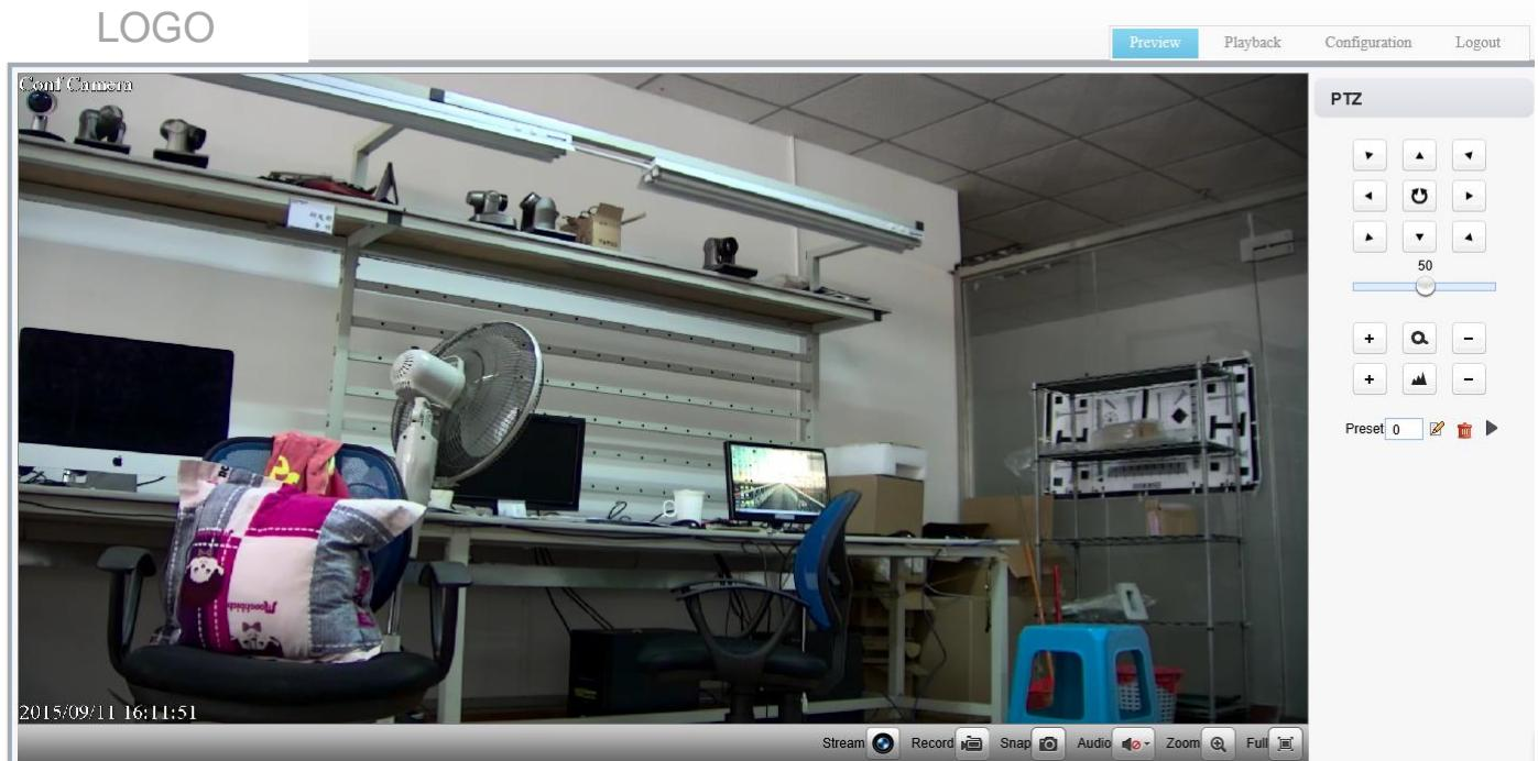
After login in the management interface it will show the default video preview interface as above picture. User can control the pan tilt, zoom, focus, record, snapshot, audio, enlarge, full screen and preset set, run and delete operations etc.
